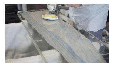
We apply a little bit of Mirka's Polarshine 25 over the cured resin and use a polishing foam pad. Once we finish, we repeat the same process but with a polishing lambswool pad. If you have followed these steps you should have right now in front of you a completely transparent surface.
